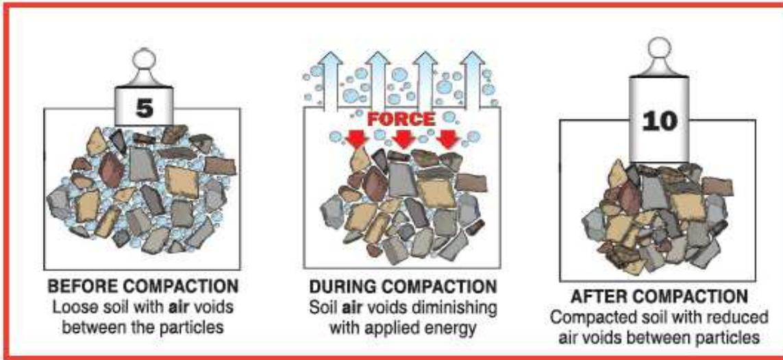
particles. The only way to change the effective compaction force is by adding or subtracting the weight of the machine. Static compaction is confined to upper soil layers and is limited to any appreciable depth. Kneading and pressure are two examples of static compaction.
