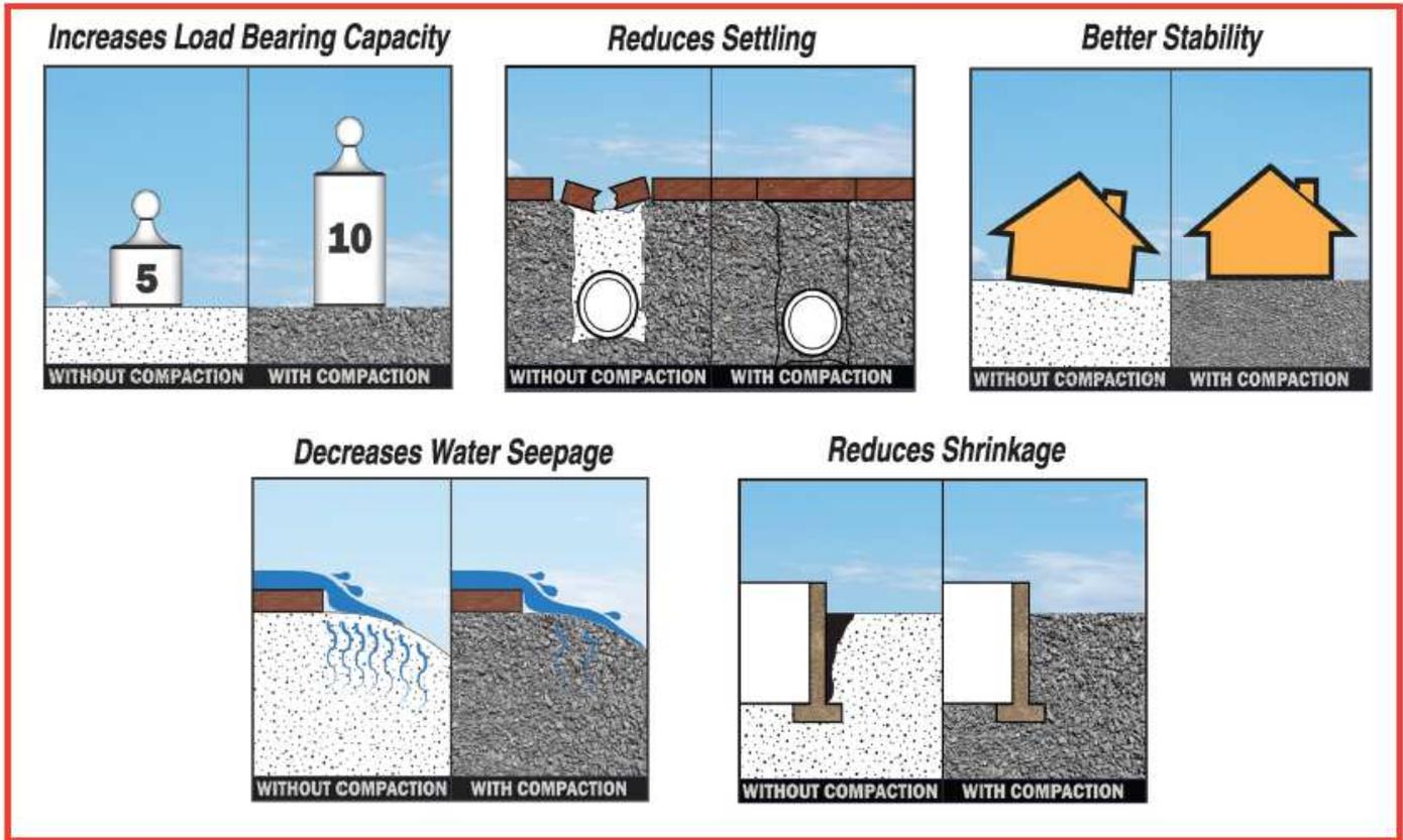
**Figure 3** — These illustrations show the results of improper compaction and how proper compaction can ensure a longer structural life, eliminating future foundation problems.
